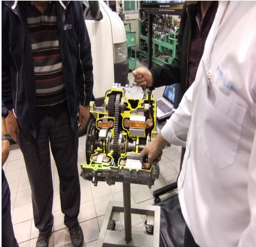
The two electric motor generators (MG1 on the left and MG2 on the right) with a power split device and drive chain between them and disc clutch plate on end where connection to petrol engine occurs. Electric motor and transmission water cooling connections visible at bottom left.
